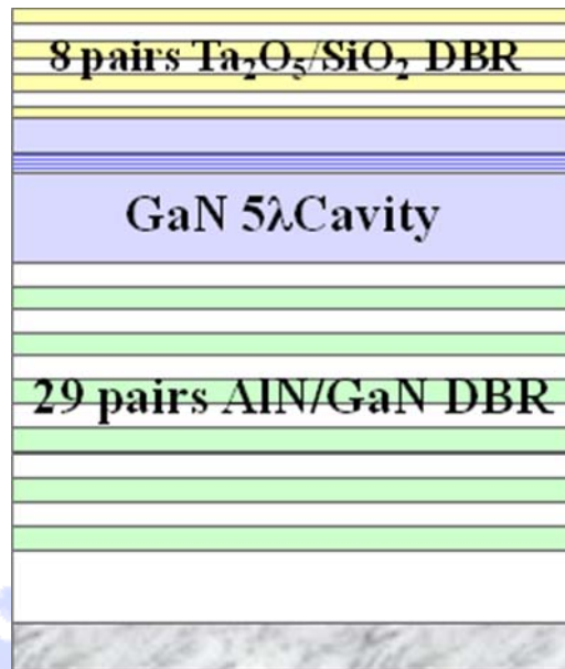
Fig 2.1 The schematic diagram of the optical pumped VCSEL structure
