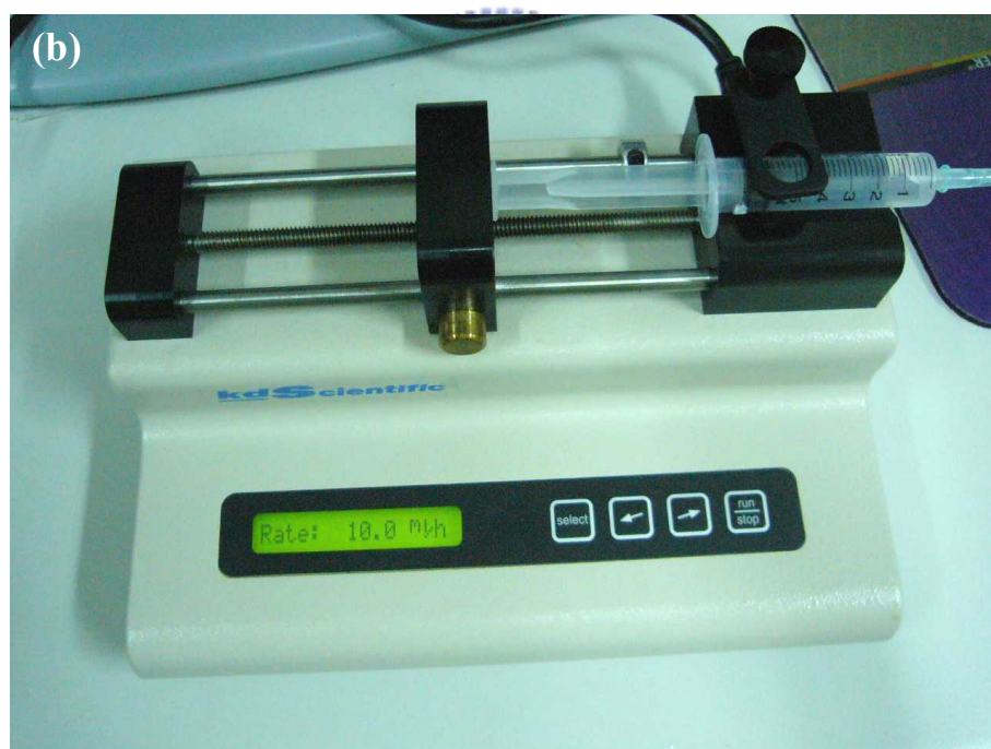
Fig. 5-5 (a) Experimental setup of the sensing measurement. (b) The micro-pump is used to inject the sample into the sensing site.
