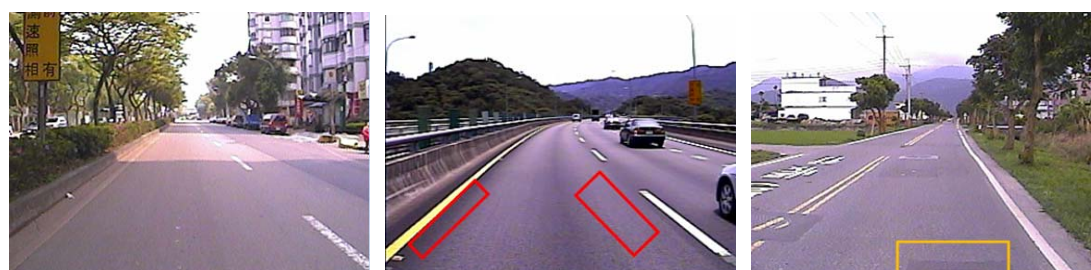
Fig. 2-4: The non-homogeneous appearance of surface causes instability of the region-based without adaptive module.
