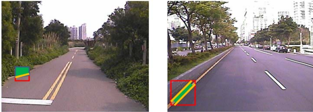
Fig. 3-12: The area around the boundary shown the red box must have specific road region ratio/non-road region ratio of the whole area. Besides, the area has the obvious difference as seen the yellow line.
