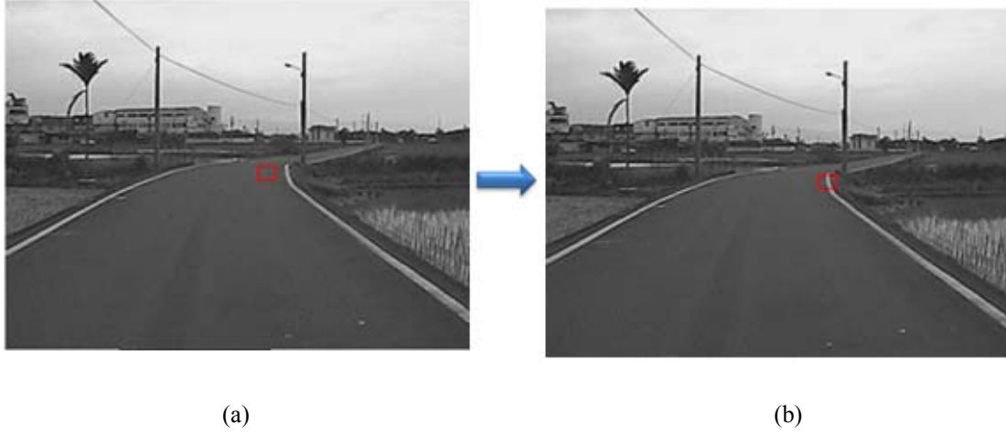
Fig. 4-10: Using the modified boundary detection solves the problem when encountering curve road boundary. The modified result is converging from (a) to (b).
