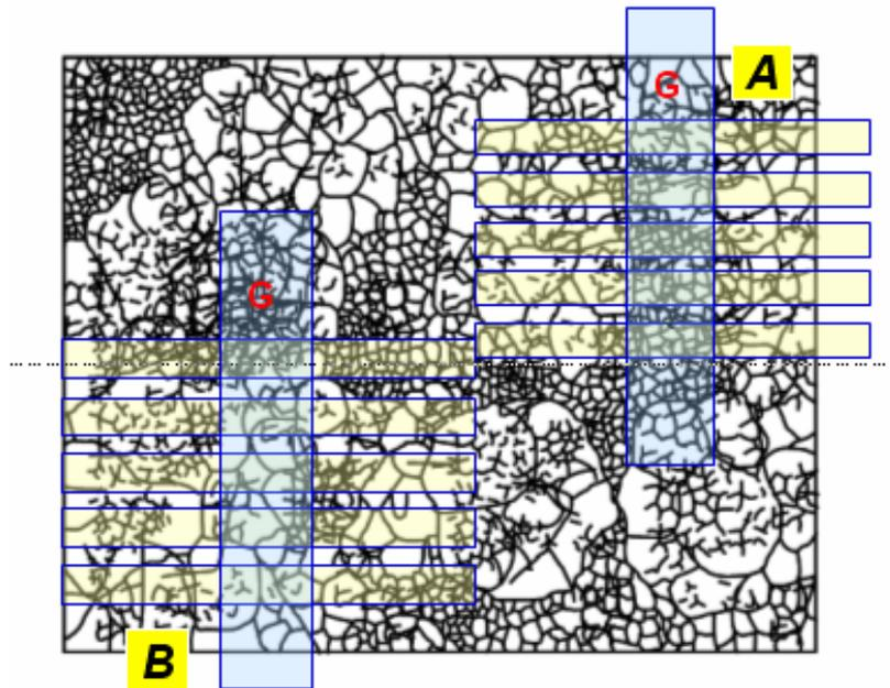
Fig. 2-19.(b) Probable distribution of relative location between devices and grains in
