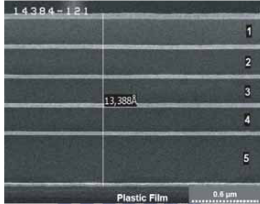
Fig. 2-10 Organic/inorganic multilayer structure from Barrix™ Systems.[4,5]
