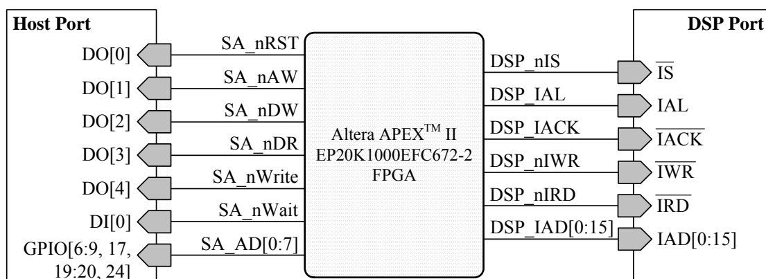
Figure 33. Functional diagram of hardware adapter
