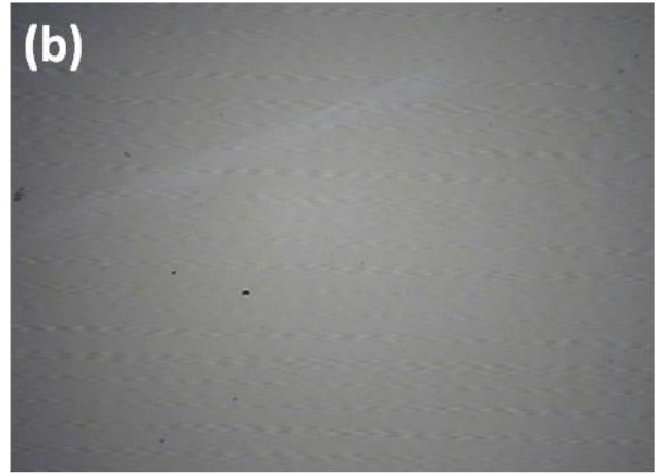
Figure 4. 14 Surface morphology of ITO/PI sample (a) as-deposited and (b) after the thermal cycling
