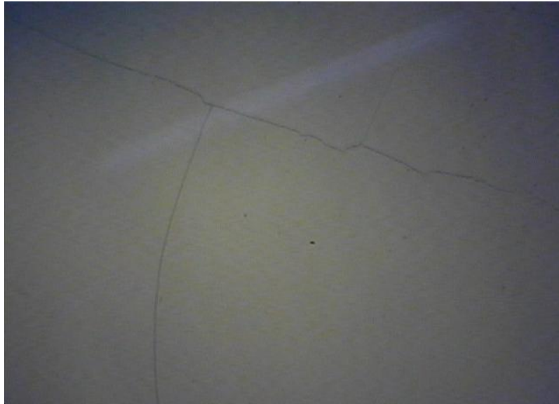
Figure 1. 1 Morphology of a cracked ITO film on PET
