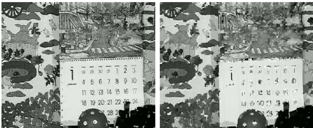
Fig. 27 mobile: left figure is our proposed predictor, 23.6dB; right figure is H.264 intra predictor, 17.9dB
