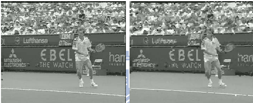
Fig. 29 Stefan: left figure is our proposed predictor, 25.9dB; right figure is H.264 intra predictor, 19.8dB
