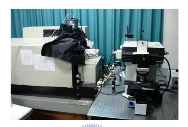
Figure 2-9 High resolution confocal Raman microscope (HOROBA, Lab RAM HR) was also applied to analyze the crystallinity of the CNTs.
