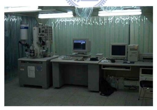
Figure 2-7 The micrographs of samples were taken by scanning electron microscope (SEM, Hitachi S-4700I).
