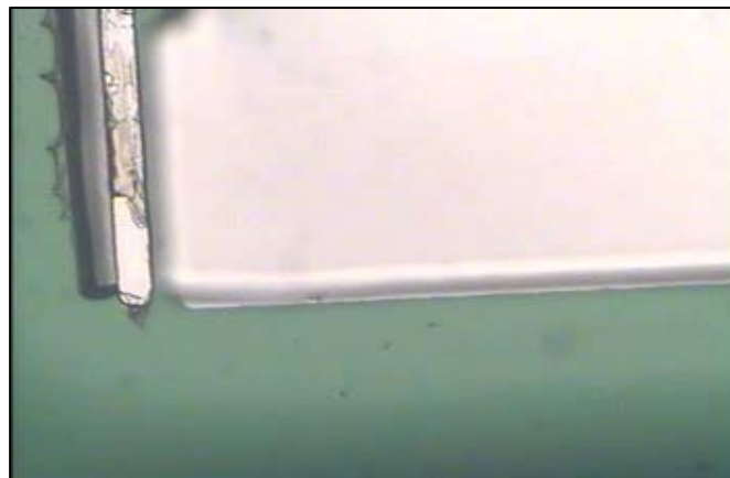
Fig.60 Overlapping parallel capacitor while applying voltage. Upper electrode moved downward by electrostatic force
