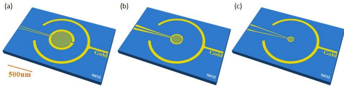
Figure 4-9 Different sizes of electrode. (a) inner diameter: 500 \mu\text{m} (b) inner diameter: 250 \mu\text{m} (c) inner diameter: 100 \mu\text{m} .
