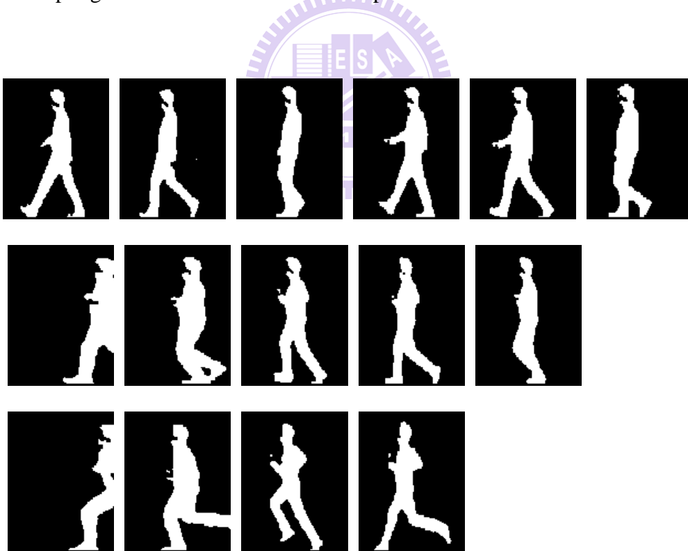
Fig. 4.5 Some essential templates use the same down-sampling rate. From top to bottom: walking, jog and running, respectively.
