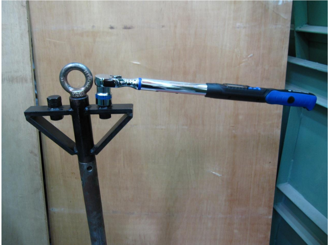
Fig. 3.13. Torque wrench are installed on the cyclic torsional loading frame (after Chen, 2011)
