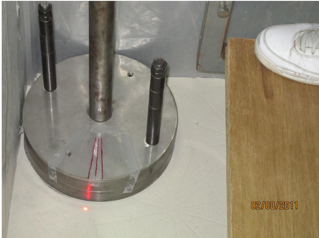
Fig. 5.17. Shear disc rotated to \theta = +5^\circ (after Chen, 2011)
