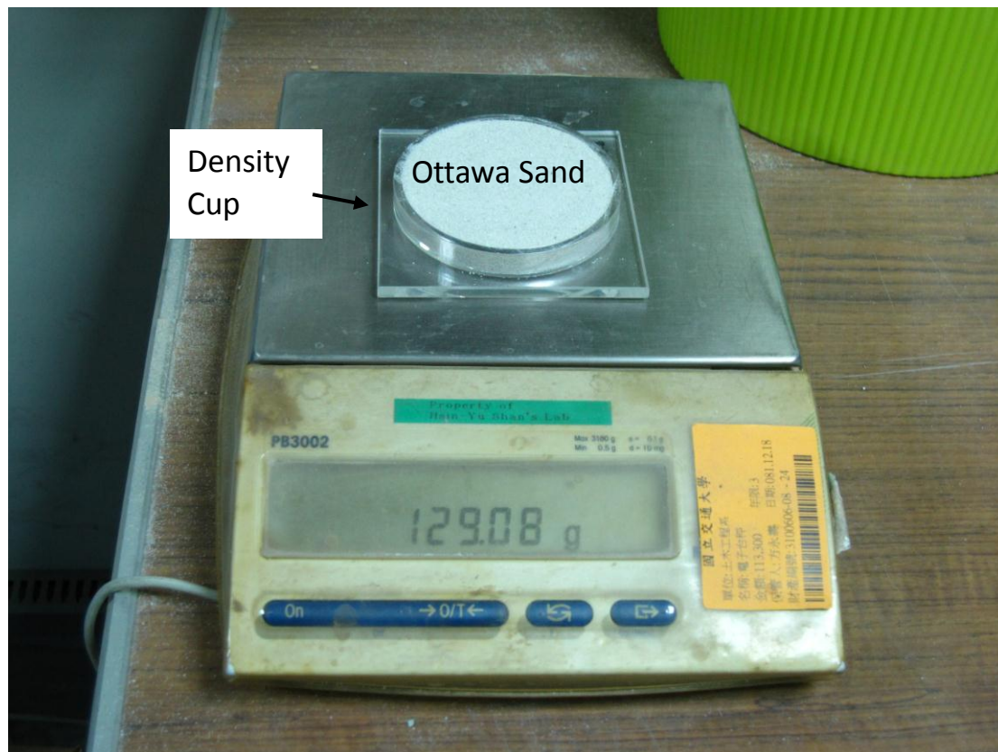
Fig. 4.11. Measurement of soil mass in density cup
