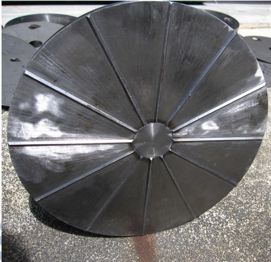
Fig. 3.5. Bottom of shearing disc with radial fins (after Chen, 2011)
