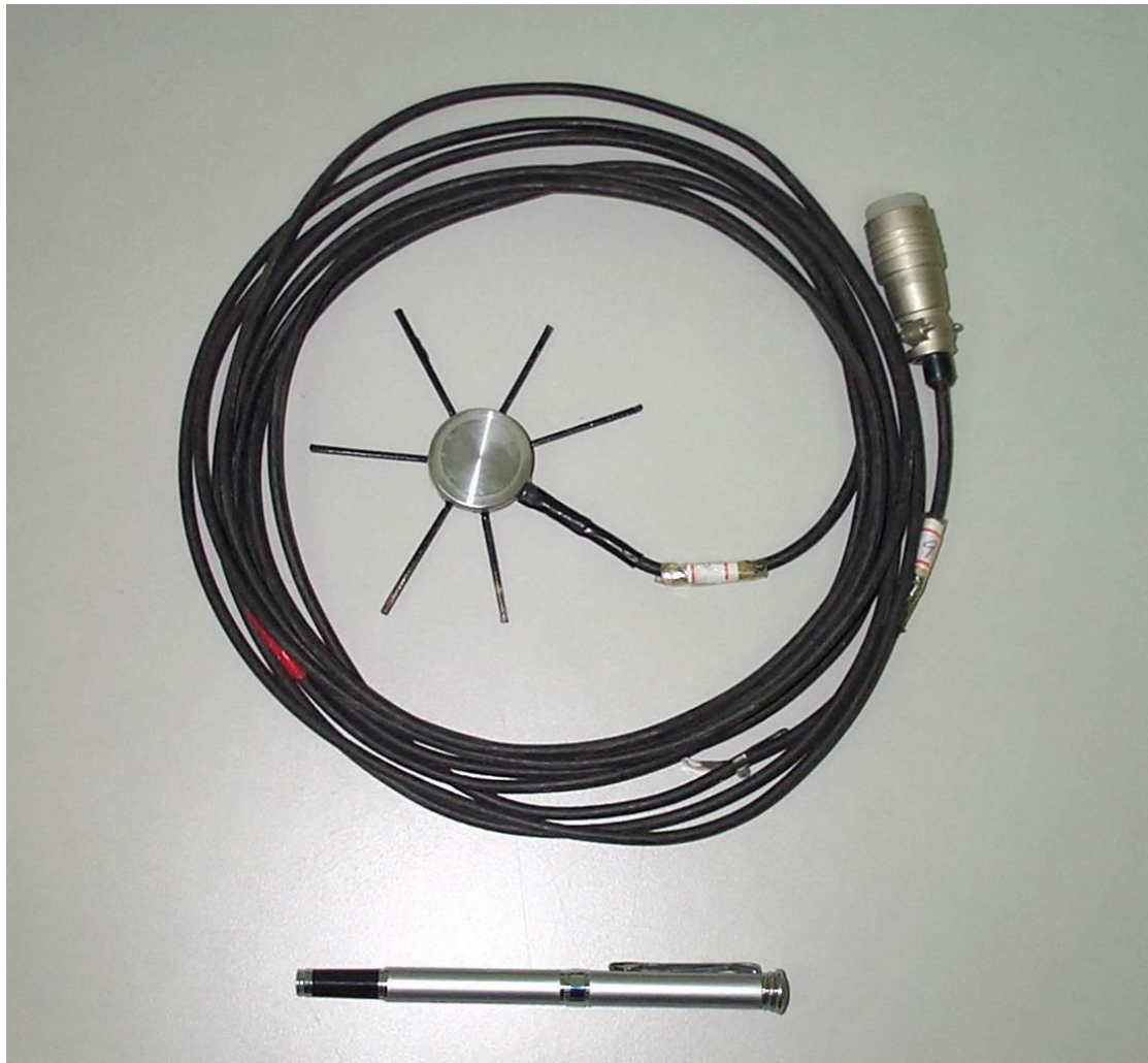
Fig. 3.2. Soil-Pressure Transducer (Kyowa BE-2KCM17) (after Chen, 2003)
