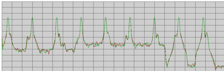
Figure 65: The spectrum of decoded audio with audio patch method corresponding to Figure 64. The zero band dithering generates the unsuitable noise floor with an excessive energy.
