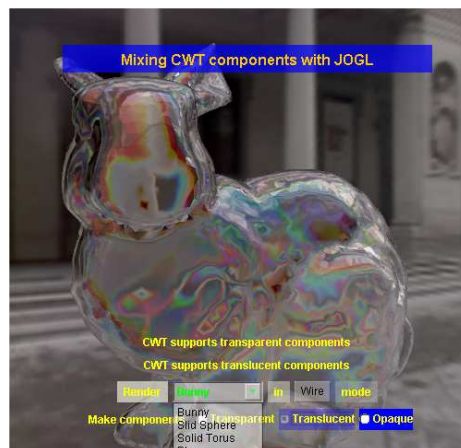
Figure 41. A shared buffer used by JOGL programs and CWT-GL, which allows translucent widgets.
