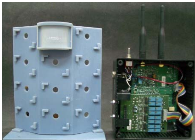
Fig.3.13 A sensor module (including a PIR detector, a Fresnel lens array, Texas Instrument micro-controller (MSP430149) and RF transceiver (TRF6901) module).
