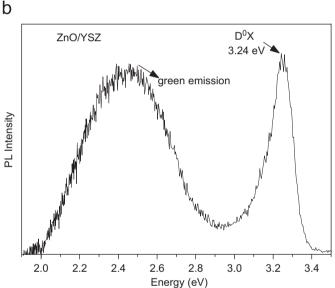
Fig. 3. Room-temperature PL spectra of ZnO layers grown on (a) GaN and (b) YSZ.
