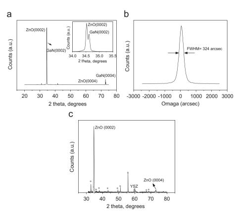
Fig. 1. (a)  $\theta$ –2 $\theta$  XRD pattern of ZnO on GaN. The inset is the enlargement of ZnO and GaN (0002) peaks; (b) (0002) rocking curve of ZnO on GaN; (c)  $\theta$ –2 $\theta$  XRD pattern of ZnO on YSZ. The peaks marked with \* are reflections from ZnO and YSZ due to the Cu–K $\beta$ , Ni–K $\alpha$  and W-L $\alpha$ <sub>1</sub> radiations from a contaminated X-ray source.
