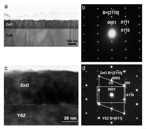
Fig. 4. (a) Cross-sectional bright-field TEM image of ZnO on GaN and (b) the corresponding electron diffraction pattern in  $[2\ \bar{1}\ \bar{1}\ 0]$  zone axis. (c) Cross-sectional bright-field TEM image of ZnO on YSZ and (d) the corresponding electron diffraction pattern in  $[1\ 1\ 0]$  zone axis of YSZ.
