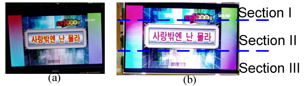
Fig. 10. (a) The power consumption of LCD panel with color filter and CCFL backlight is larger than 5W. (b) The power consumption of the color filter-less LCD panel with the proposed RGB backlight driver is about 2-3W.
