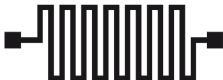
Fig. 1. Configuration of spiral silver metal lines screen-printed on alumina substrate for the resistivity measurement.
