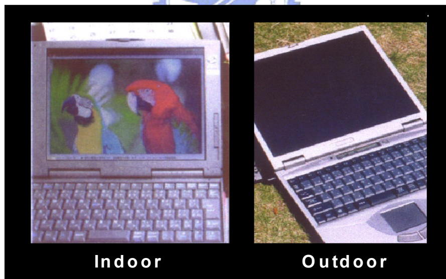
Fig. 1-4. Demo photos of a transmissive type LCD at the indoor and outdoor environment.
