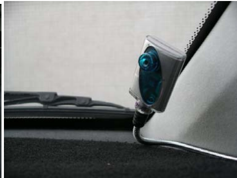
Fig. 17. The USB camera mounted behind the right front windshield.
