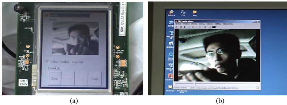
Fig. 24. (a) The real-time image is recorded by OMAP5912. User can review the image from (b) by Internet.
