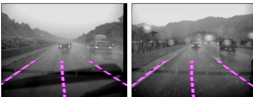
(a) Interference of windshield wipers. (b) Interference of strong light in rainy days. Fig. 21. Detection in the front view.
