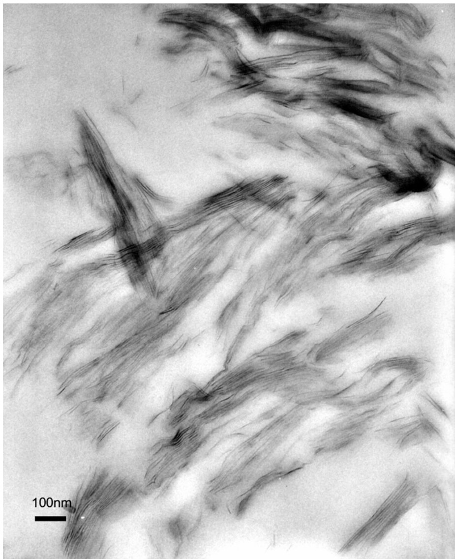
Figure 2.2 TEM micro-photos for the epoxy/organoclay nanocomposites ((a) 50,000 magnification).
