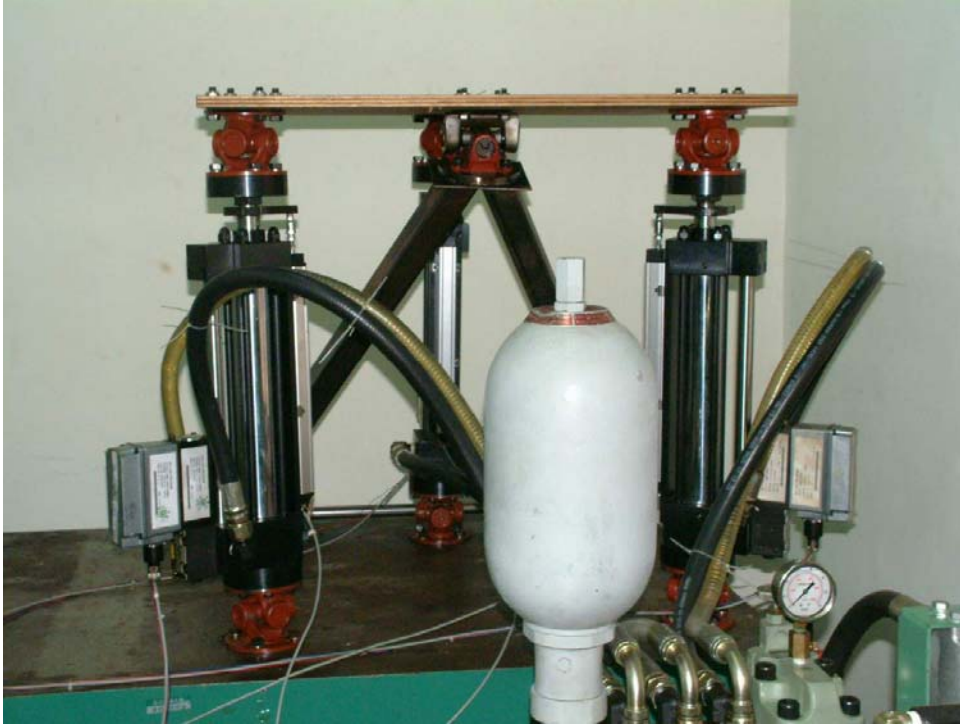
Fig. 2.1. (b) Hydraulic motion platform
