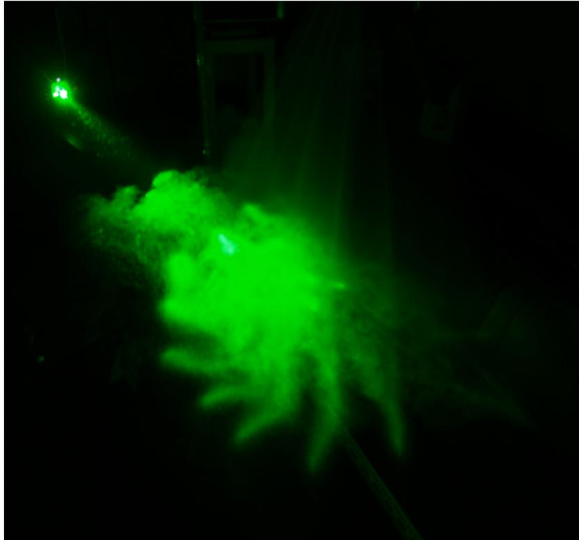
Fig. 4.30 Water mist distribution picture for  $P=30 \text{ Kg/cm}^2$ .
