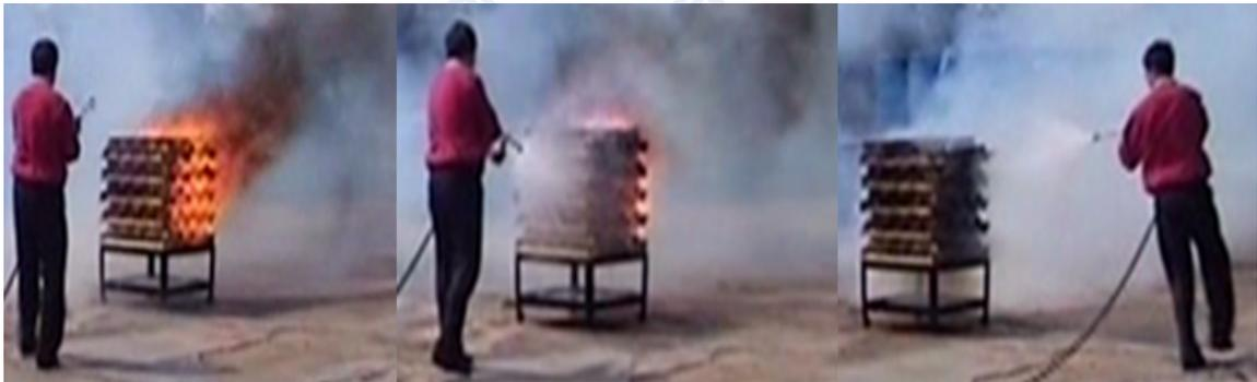
Fig. 4.1 Pictures of Class A fire test
