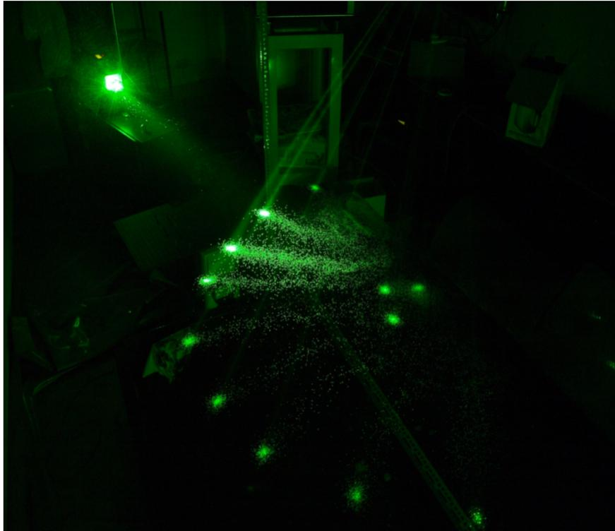
Fig. 4.26 Water mist distribution picture for  $P=10 \text{ Kg/cm}^2$ .
