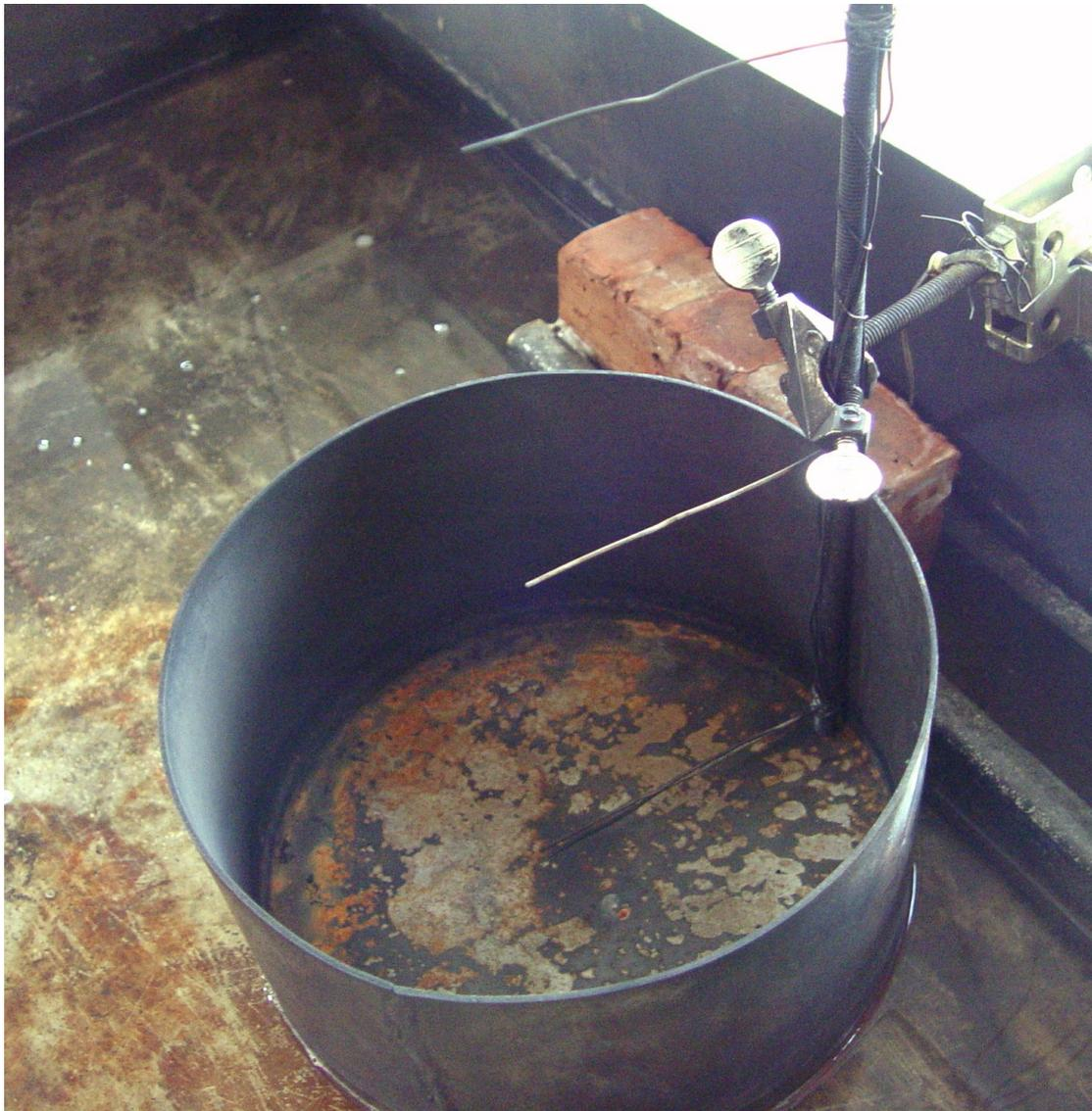
Fig. 2.5. The picture of thermocouple tree
