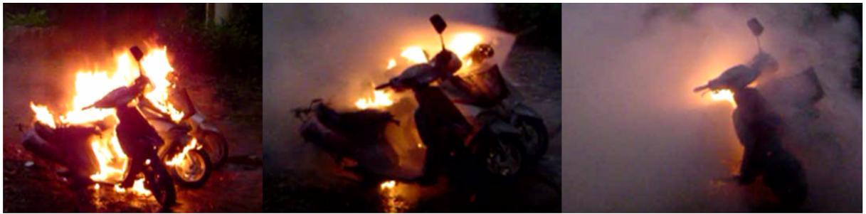
Fig. 4.3 Pictures of motorcycles fire test
