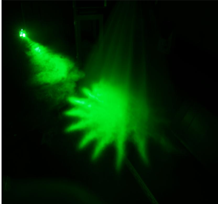
Fig. 4.32 Water mist distribution picture for  $P=40 \text{ Kg/cm}^2$ .
