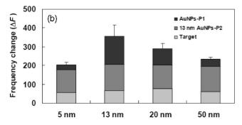
**Figure 2.** The enhancement of detection signal by different sizes of AuNP probes. (a) In the experiments, 5, 13, 20 and 50 nm AuNPs–DENV2-P2 were used as the first layer and 13 nm AuNPs–DENV2-P1 as the second layer enhancers. (b) In the experiments, 13 nm AuNPs–DENV2-P2 were used as the first layer and 5, 13, 20 and 50 nm AuNPs–DENV2-P1 as the second layer enhancers. Each value was derived from three independent detections and the error bars mean SD.
