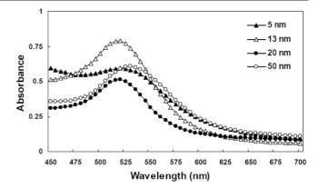
**Figure 1.** UV–vis absorption spectra of the AuNPs with different diameters. Four sizes of AuNPs with diameters of 5, 13, 20 and 50 nm were measured by a UV–vis absorption spectrophotometer, and they exhibited an absorption maximum at 520–540 nm arising when the AuNPs exhibit noticeable absorption and scattering from the colloid gold localized surface plasmon resonance.
