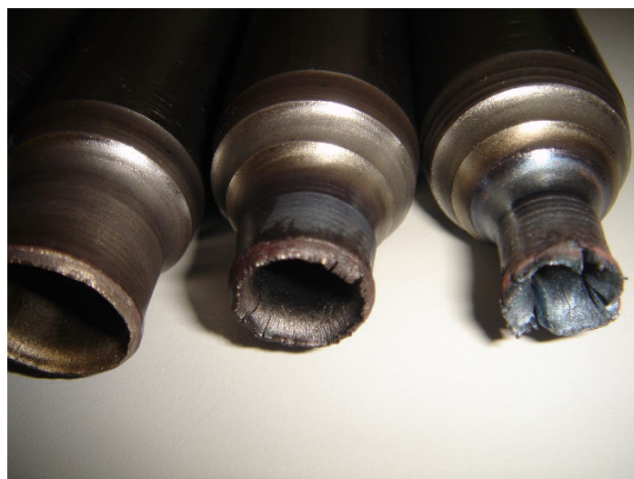
Figure 1.6 Fracture after spinning at room temperature
