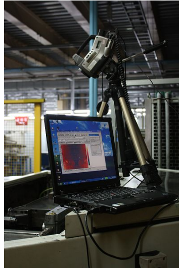
Figure 3.5 Infrared camera (FLIR ThermoCAM-S65)
