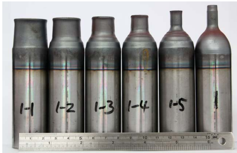
Figure 3.10 Six steps of spun tubes
