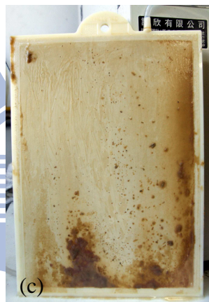
Figure 4.9. Pictures of the membranes fouled at different SRTs: (a) 10 days; (b) 30 days and (c) 60 days. All these pictures were taken when the TMP reached -60 kPa.
