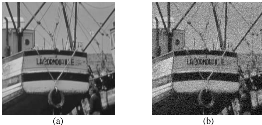
Fig. 4.5. (a) Original “Boats” image; (b) Noisy image of “Boats” with Gaussian noise only of \sigma = 20 .
