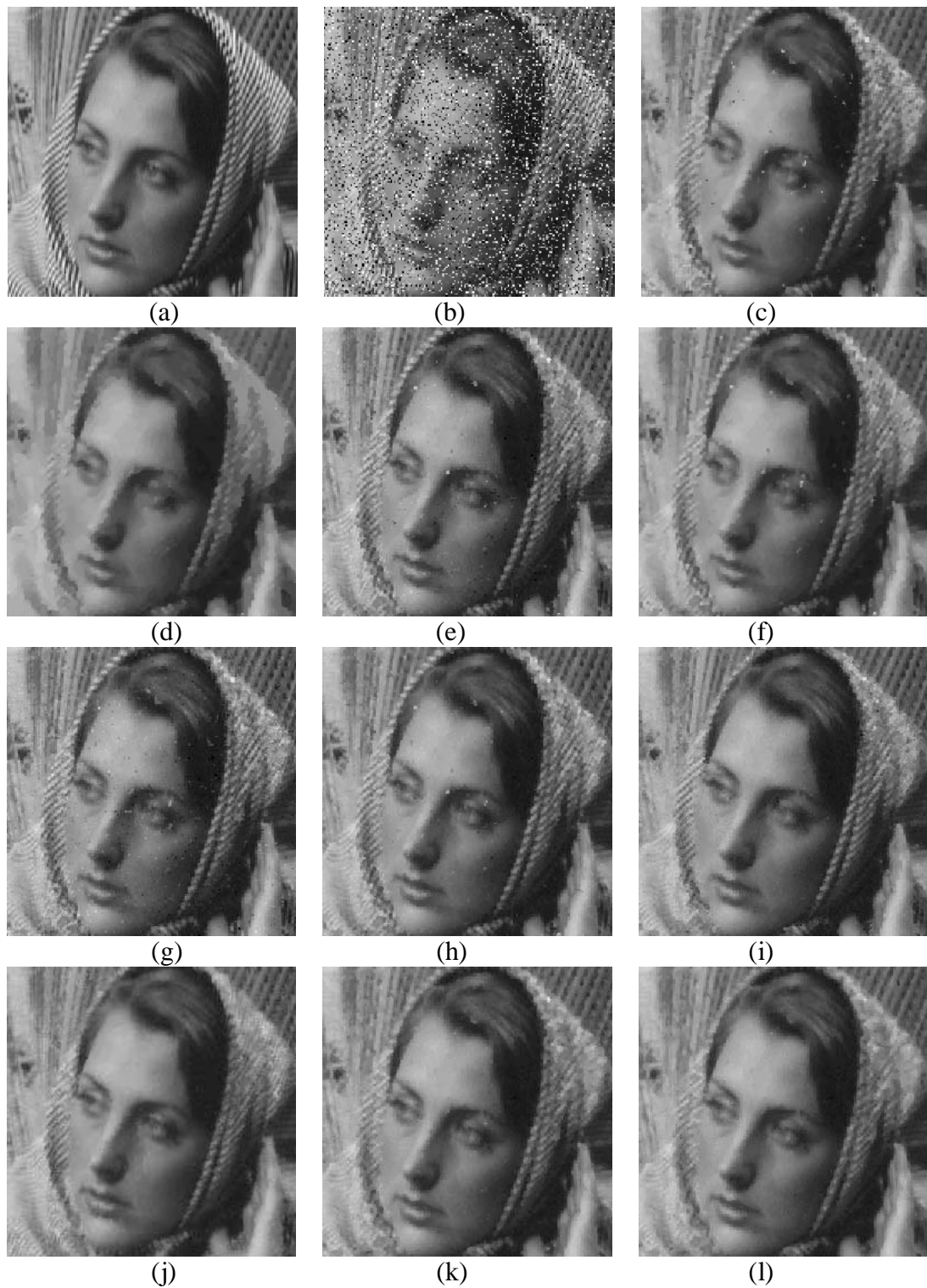
Fig. 3.19. (a) Original image; (b) Barbara with 25% of random-valued impulse noise; (c) the 3 \times 3 standard median filter; (d) the 3 \times 3 recursive median filter; (e) the recursive tri-state median filter with threshold = 25; (f) optimal weighted median filter; (g) Li's edge preserving method with threshold = 32; (h) PBM filter; (i) Zhang's fuzzy techniques; (j) Trilateral filter; (k) 1st step of the proposed method; (l) The proposed two-step method.
