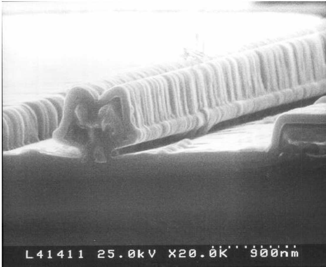
Figure 3-2 The SEM image of the T-shaped gate.
