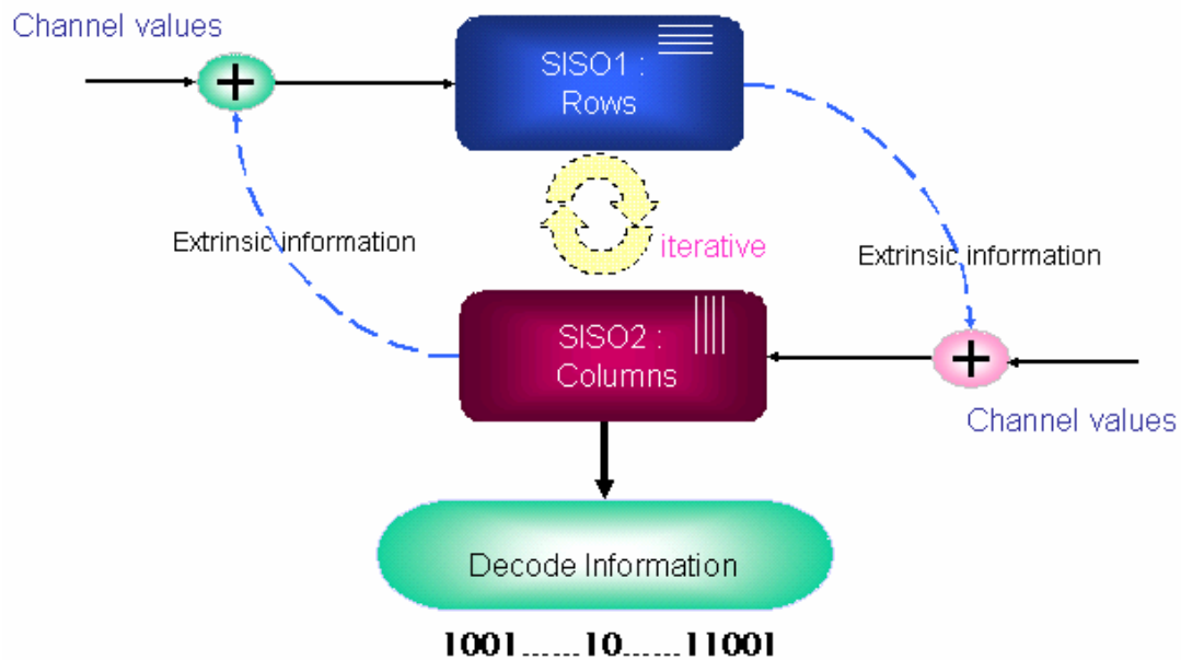
Figure 2.4: The flow diagram of iterative decoding algorithm
