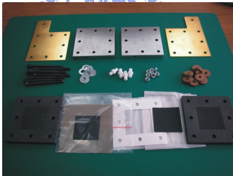
Fig. 2.12 All components of PEMFC
