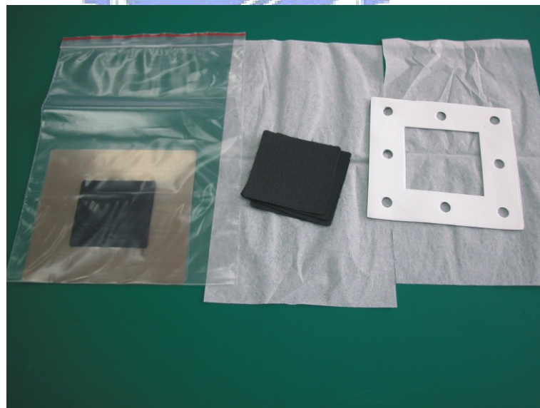
Fig. 2.8 MEA, GDL, and gasket
