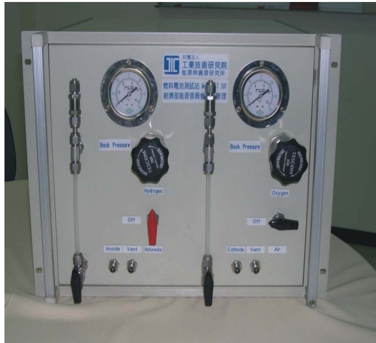
Fig. 2.5 Gas pipelines controller
