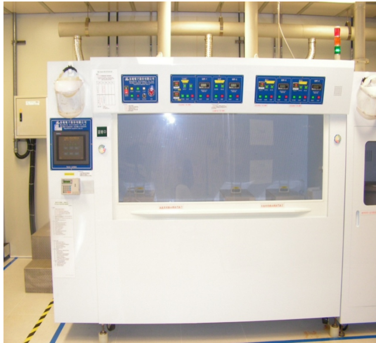
Fig. 2.15 RCA cleaning (Wet bench)
