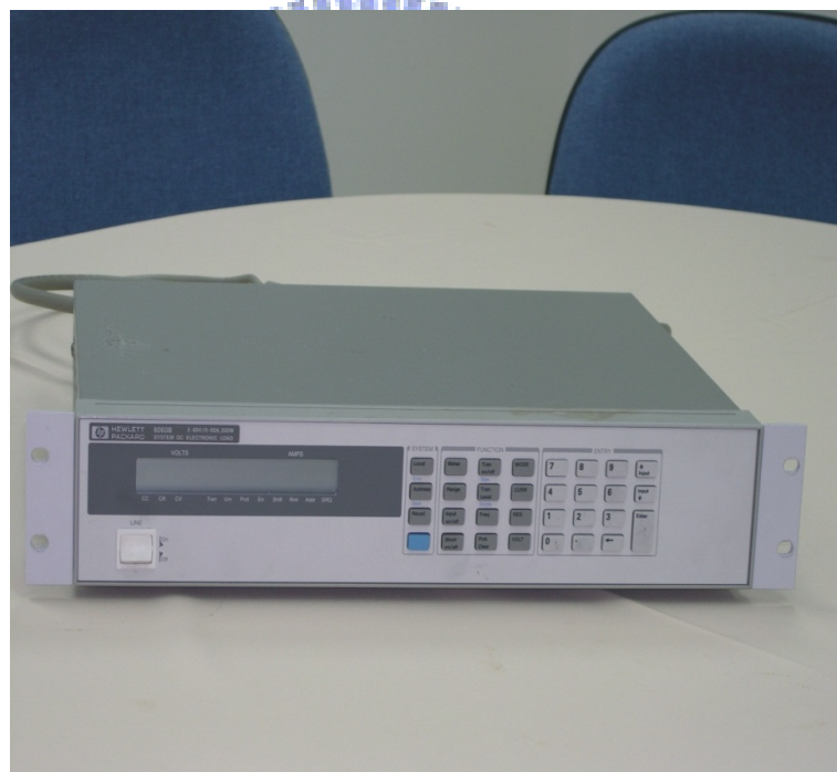
Fig. 2.2 HP 6060B electrical load
