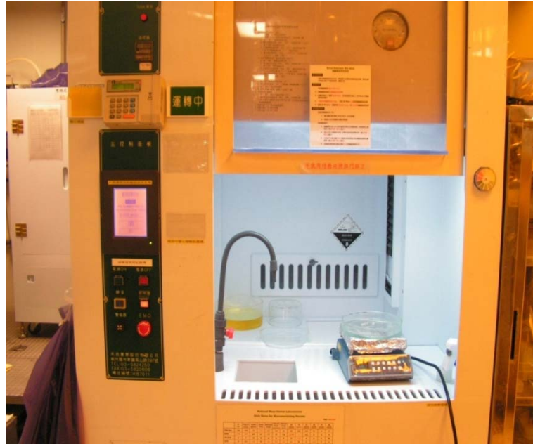
Fig. 2.19 Wet etching chemical hood
