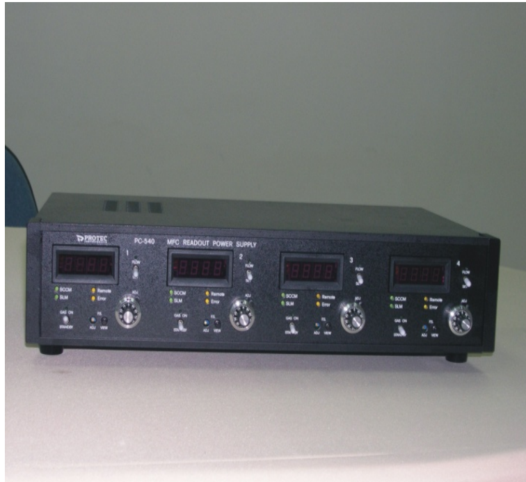
Fig. 2.3 MFC readout power supply
