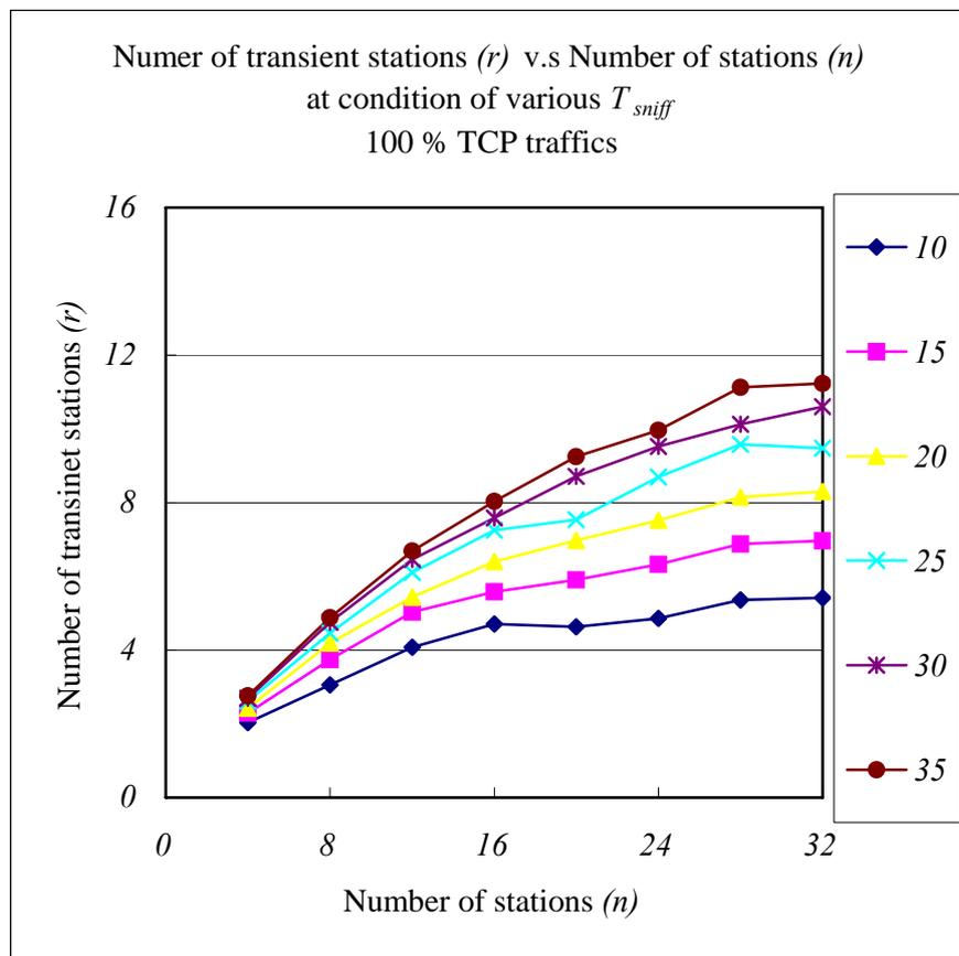
Figure 4.3 Number of transient stations v.s. number of stations in EDCA with 100% TCP nodes.
