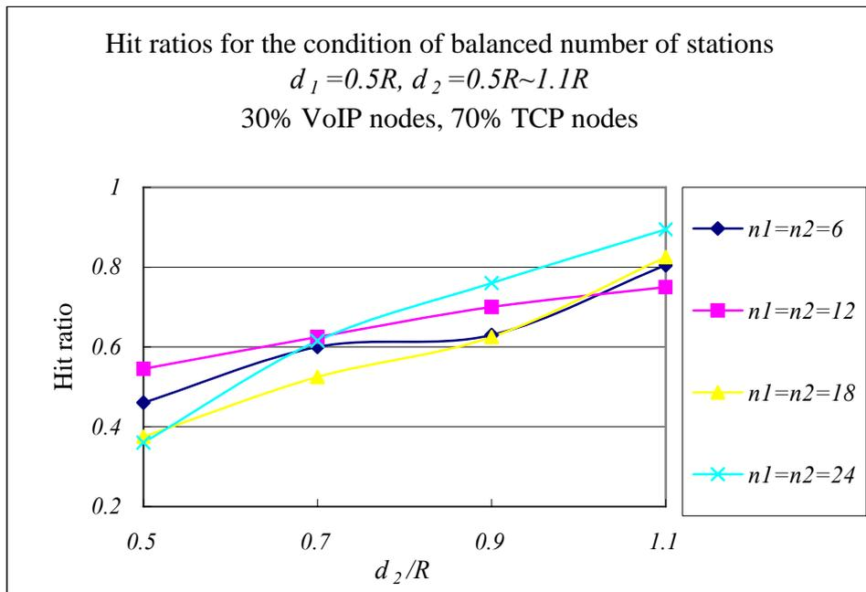
Figure 4.4 Hit ratios v.s. distances in balanced number of stations in EDCA WLAN of 30% VoIP nodes and 70% TCP nodes.
