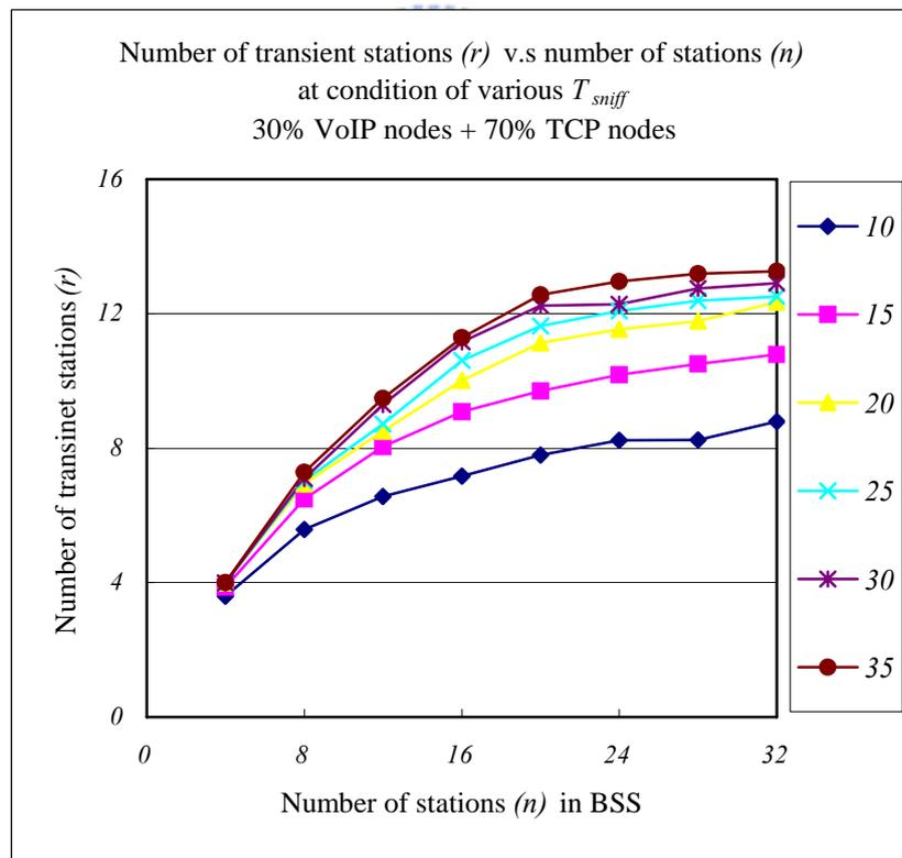
Figure 4.2 Number of transient stations v.s. number of stations in EDCA of 70% TCP and 30% VoIP nodes.
