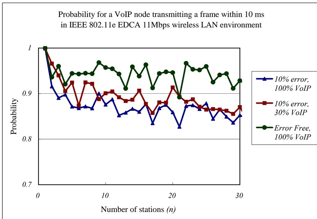
Figure 4.8 Probability to send a frame in 10 ms v.s. number of stations in 11 Mbps EDCA wireless LAN.
