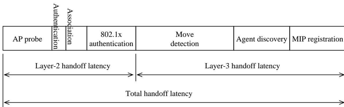
Figure 2.1 Overall latency in a layer-2 and layer-3 handoff
