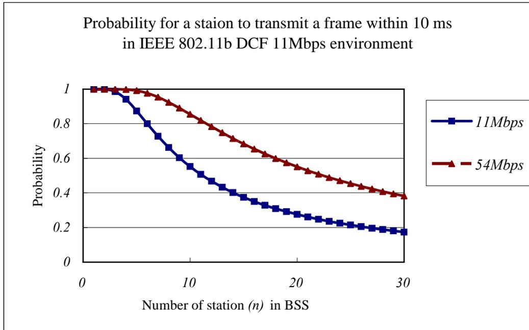
Figure 3.12 Probability to transmit a frame in 10 ms v.s. number of stations in a BSS.
