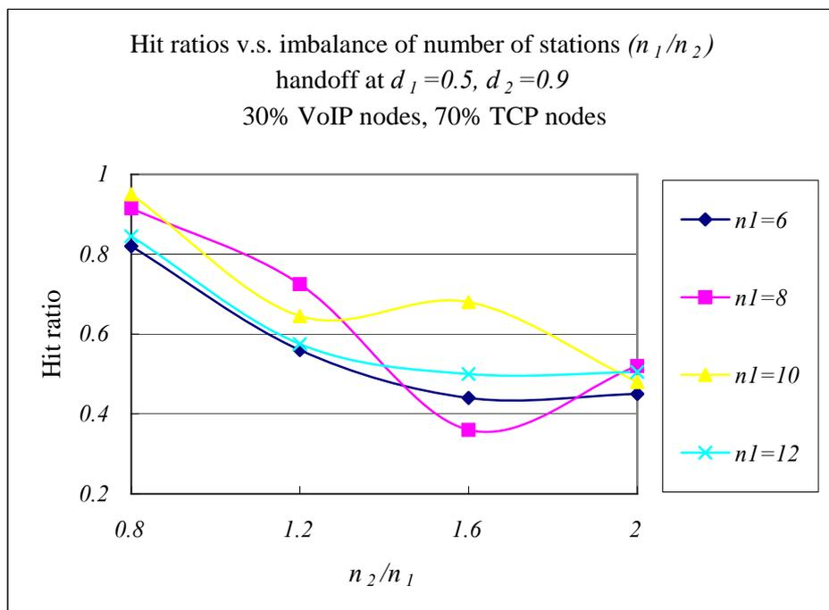
Figure 4.6 Hit ratios v.s. imbalanced number of stations in EDCA of 30% VoIP nodes and 70% TCP nodes.
