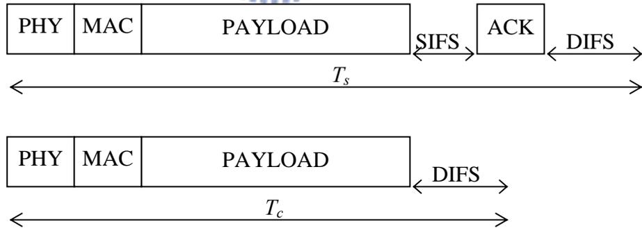
Figure 3.6 Definition of  $T_s$  and  $T_c$ , slot time of transmission with success and collision.
