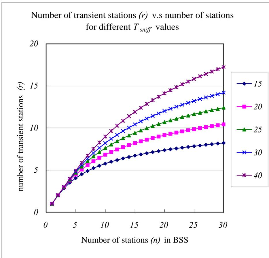
Figure 3.7 Number of transient stations ( $r$ ) v.s. number of stations ( $n$ ) for different  $T_{sniff}$  values.
