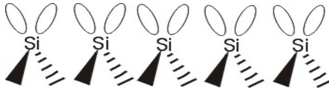
Fig. 1.2 The side view of an ideal Si(100) surface. Each silicon atom has two valence bonds and two dangling bonds.
