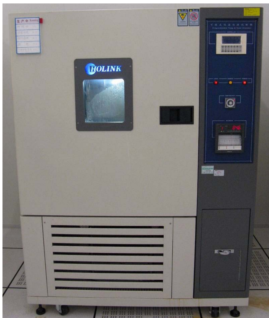
圖3-7 Temperature & Humidity Storage Test Machine
