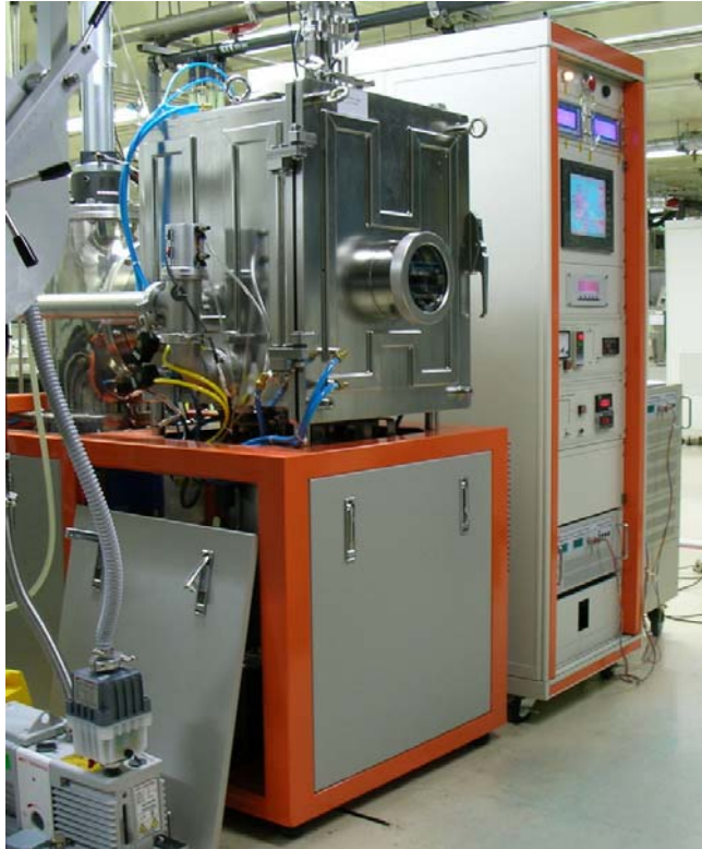
Fig. 3-6. Thermal coater system for OLED fabrication.
