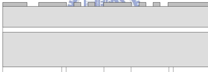
(c) Front side mask patterning by double side photolithography
