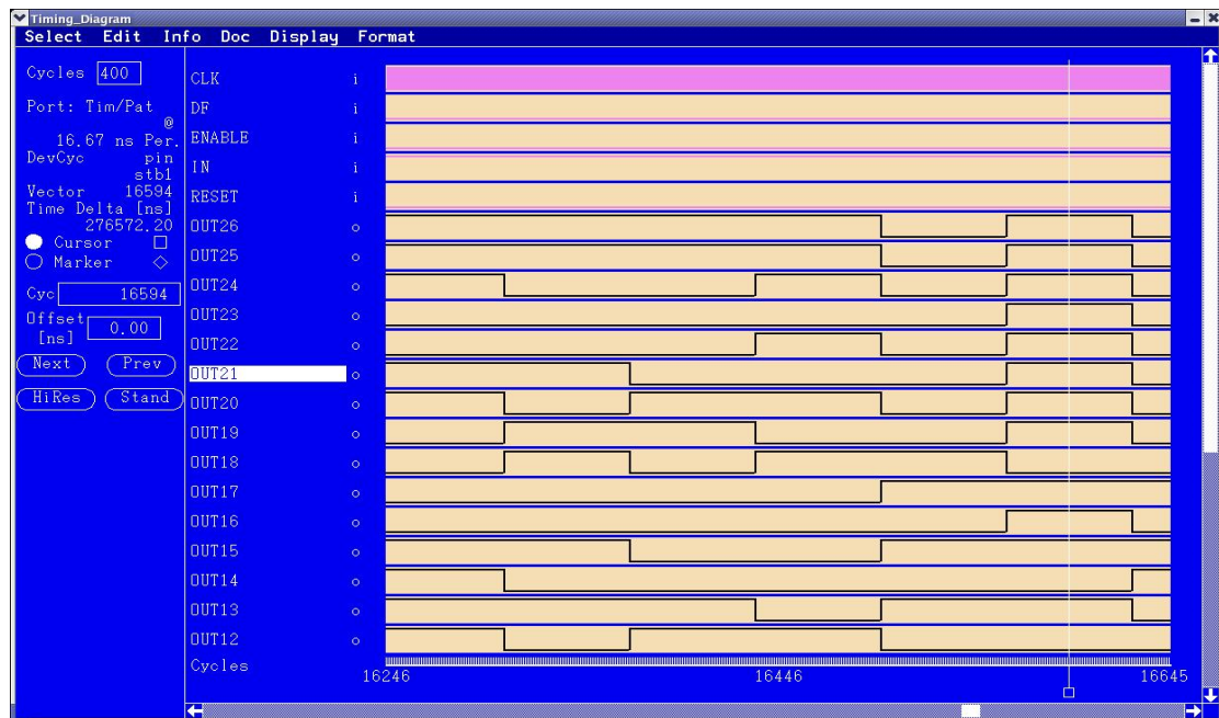
Figure 4.13 Timing diagram (decimation ratio 64) plotted by Agilent 93000
