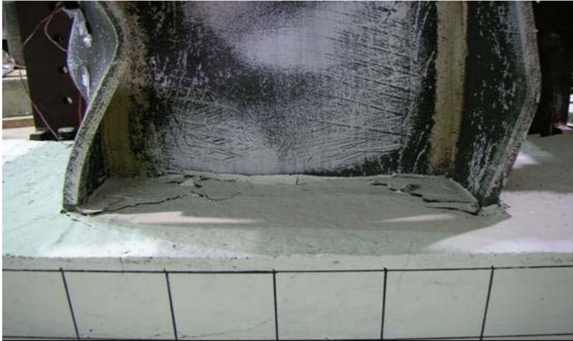
(b) 試體 SRC2-VR1.15 位移  $11\Delta_y$  時 (Story Drift Angle  $\theta_t=5.25\%$  , Beam Plastic Rotation  $\theta_{bp}=4.44\%$ ) 柱上方鋼梁附近混凝土之開裂情況
