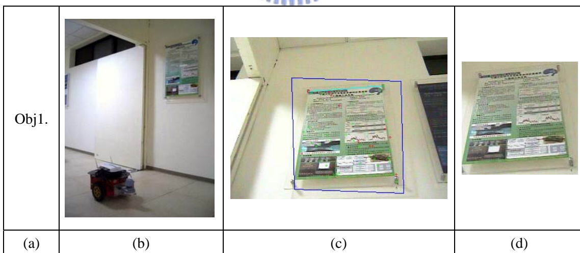
Figure 8.3 The experimental result of object monitoring and navigation path correction. (a) Monitored object labels. (b) The vehicle monitors the monitored objects. (c) The matching result and the horizontal line used for path correction. (d) The image of learned monitored objects.
