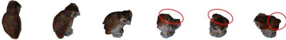
Fig. 17. The results of the automatic initial segmentation corresponding to the image sequence shown in Fig 16. The three images on the left show the segmentation results that should be selected for the 3D reconstruction, while the others shows results that should be excluded and refined in the next run. The red circles denote the noticeable segmentation errors in each image.
