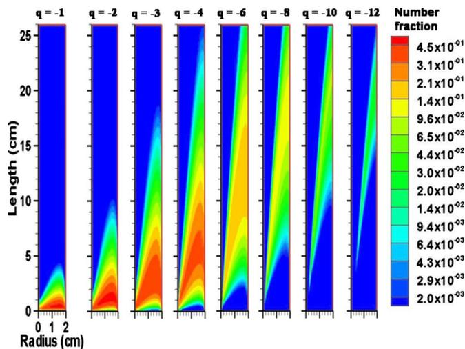
FIG. 3. (Color online) Distribution of negatively charged nanoparticles with diameter of 65 nm and charges  $q = -1, -2, -3, -4, -6, -8, -10, -12$ . The wire-tube corona charger is 2 cm in radius and 26 cm in length with  $\varphi_w = -9.5$  kV and  $I = 19.2 \mu\text{A cm}^{-1}$ . Mean air flow speed in the tube is  $2 \text{ m s}^{-1}$ .
