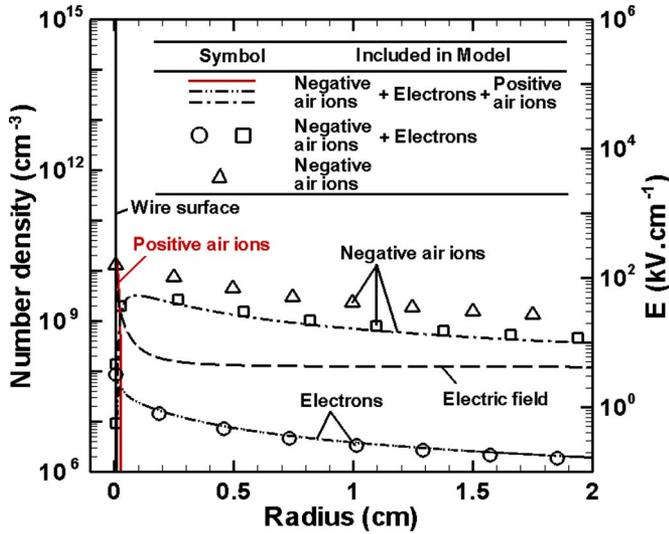
FIG. 1. (Color online) Distribution of electric field, electrons, and positive and negative ions ( $\varphi_w = -9.5$  kV and  $I = 19.2 \mu\text{A cm}^{-1}$ ). The wire-tube corona charger is 2 cm in radius submitted at  $\varphi_w = -9.5$  kV and  $I = 19.2 \mu\text{A cm}^{-1}$ .
