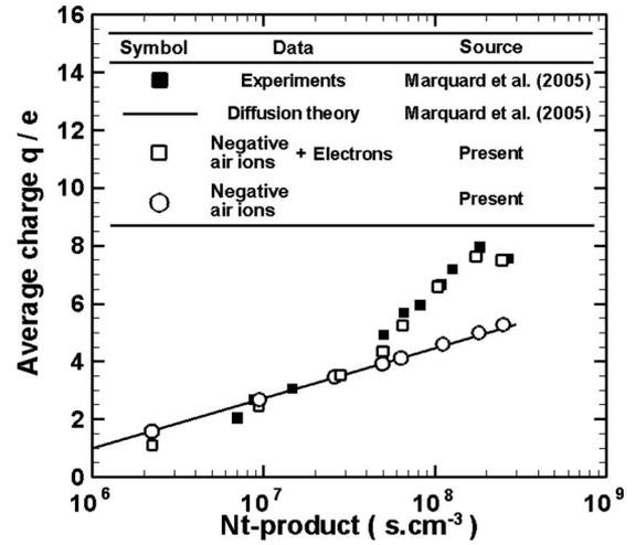
FIG. 2. Average charge carried by nanoparticles with diameter of 65 nm as a function of the  $Nt$  product. The wire-tube corona charger is 2 cm in radius and 26 cm in length. Mean air flow speed in the tube is  $2 \text{ m s}^{-1}$ .
