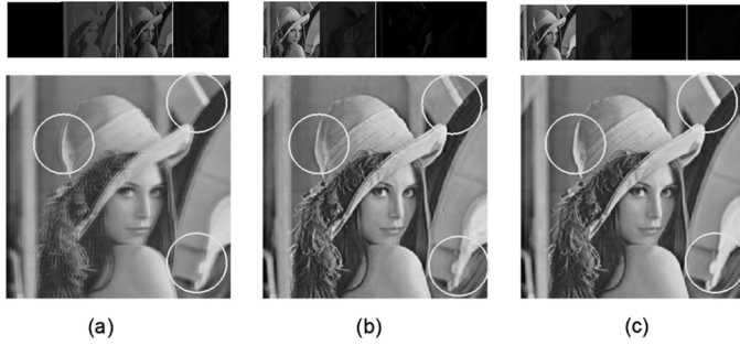
Fig. 2. Simulated CBU images of Lena in three conditions of: (a) none, (b) white, and (c) proposed D-field.
