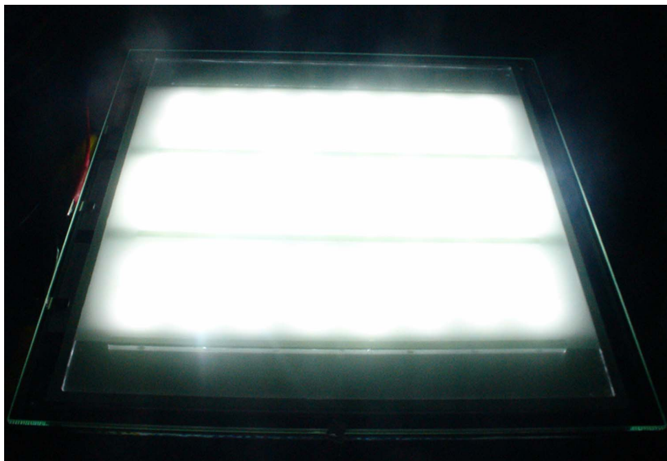
Fig. 2. Photograph of the 14-in NTL while igniting the plasma at 260 V in 50 torr of pure xenon gas.
