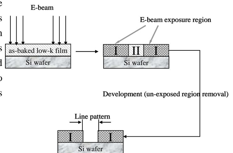
Figure 1 Proposed e-beam lithography process for the fabrication of damascene structure.
