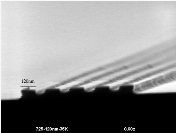
Figure 6 The SEM cross section image of dense pattern lines of e-beam exposed MSZ film after development.
