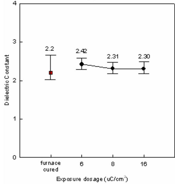
Figure 8 The dielectric constant of e-beam exposed POSG films at different doses with furnace annealing process.
