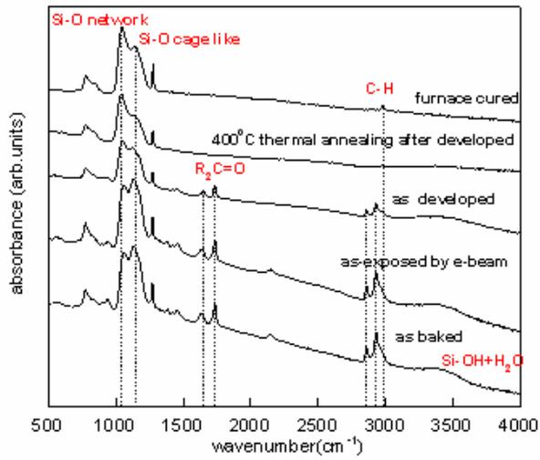
Figure 10 The FTIR spectra of POSG films with e-beam exposure and followed by development and post-thermal annealing treatments.
