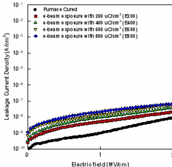
Figure 2 The leakage current of e-beam exposed MSZ is compared to that of traditional furnace cured one.
