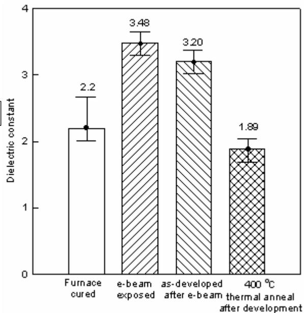
Figure 13 The dielectric constant of e-beam exposed POSG films with  $8 \text{ uC/cm}^2$  dosage after undergoing various treatment.
