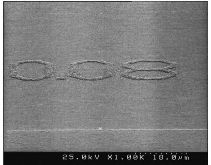
Figure 9 The SEM image of patterned wafer after e-beam curing and development processes without post-exposure annealing.
