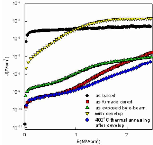
Figure 12 The leakage current density of e-beam exposed POSG films with  $8 \text{ uC/cm}^2$  dosage after undergoing various treatment.
