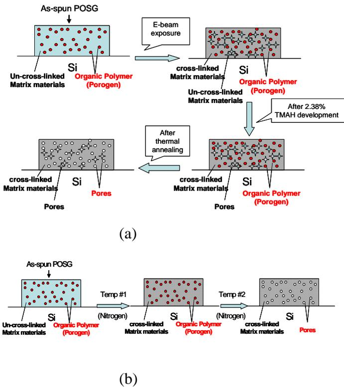
Figure 11 The proposed model for the decrease of dielectric constant on the e-beam exposed POSG after development and subsequent thermal annealing processes (a) e-beam direct patterning process (b) traditional furnace curing process.
