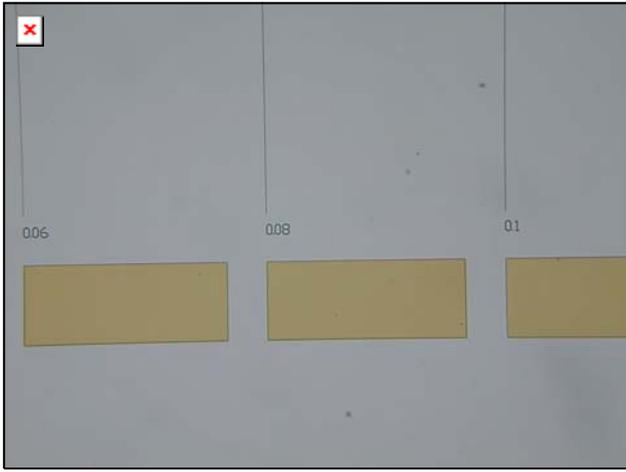
Figure 5 The optical image of single line pattern of e-beam exposed MSZ film after development.
