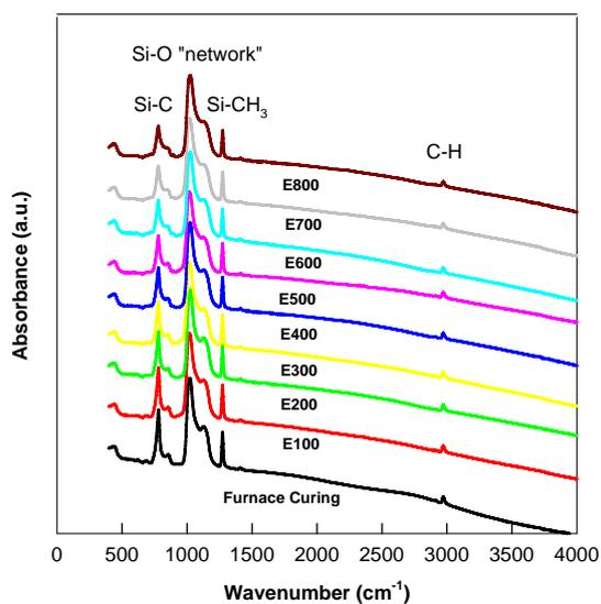
Figure 3 The FTIR spectra of e-beam exposed MSZ with different doses after thermal annealing.
