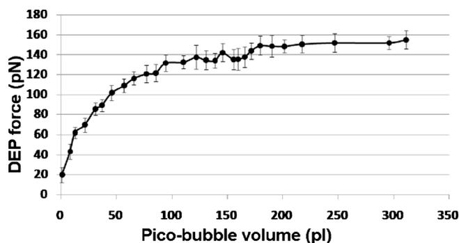
FIG. 4. (Color online) The relationship between light-induced driving force and picobubble volume. The ac voltage of 10 Vpp at 10 kHz is applied between the top and bottom ITO glass.
