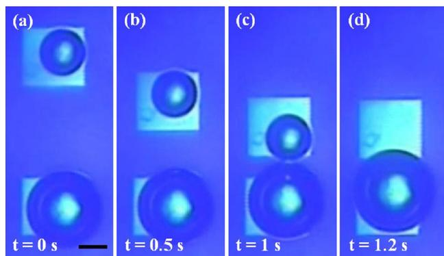
FIG. 2. (Color online) The bubble is dragged by following the trajectory of the moving light square. The light-induced driving force drags a 50 pl volume bubble to fuse another 220 pl bubble. The scale bar is 30  $\mu\text{m}$ . (enhanced online, bubbles\_manipulation.mov). [URL: <http://dx.doi.org/10.1063/1.3580760.1>]
