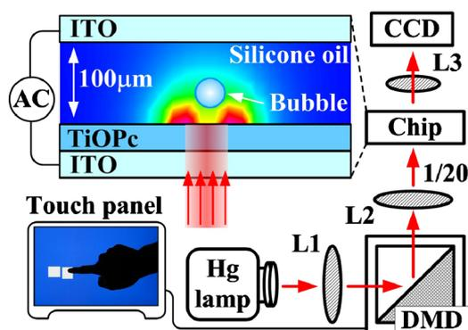
FIG. 1. (Color online) Schematic diagram of the optical system setup for our touch-panel-based light-driven optoelectronic-mechanism chip. The light-induced electric field generates appropriate force to trap the picobubble suspended in silicone oil toward the illuminating area.
