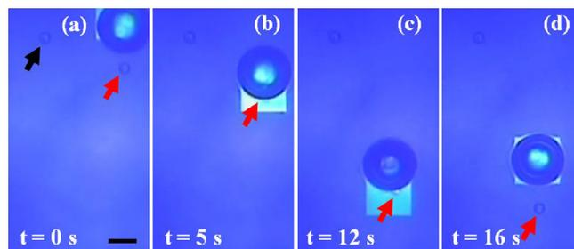
FIG. 3. (Color online) A 15  $\mu\text{m}$  diameter bead indicated with the arrow is manipulated via the optically driven picobubble. The scale bar is 35  $\mu\text{m}$ . (enhanced online, bead\_manip\_via\_picobubble\_tweezer.mov). [URL: <http://dx.doi.org/10.1063/1.3580760.2>]
