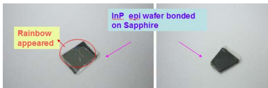
Figure 3 (a): Samples without channels after wafer-bonding.
