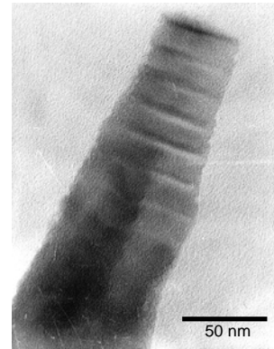
Fig. 2 Transmission electron micrograph of a single \text{In}_{0.3}\text{Ga}_{0.7}\text{N}/\text{GaN} MQWs nanorod.
