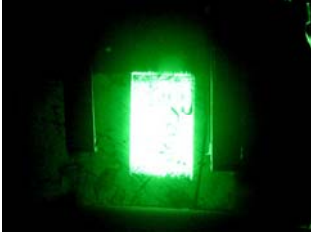
Figure 4. Emission image at applied field 5.5 V/μm for diode testing
