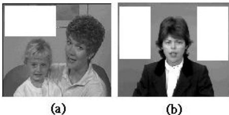
Fig. 3. Image areas used to estimate the true camera noise variance for (a) Mother-and-Daughter and (b) Claire sequences.
