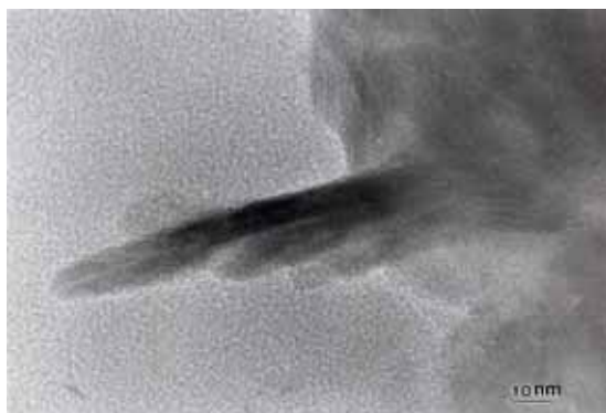
Fig. 7 High-resolution lattice fringes in the needlelike particle of CDHA crystal.
