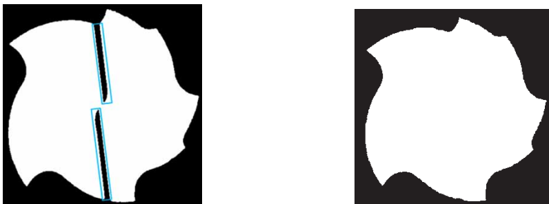
Figure 13. Two end gashes of an original fishtail. Figure 14. Filled fishtail (from Figure 13).
