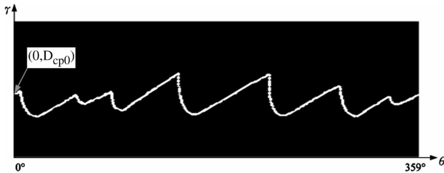
Figure 17. Centroidal profile of the boundary pixels of a fishtail with respect to the centre of the fishtail.
